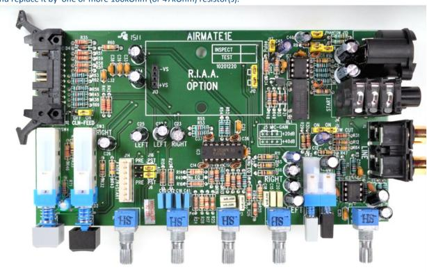
Now remove all the chips from that faulty PCB and put power again on the pcb by turning on the power supply of the Airmate. Now measure the power supply before and after this 100kOhm resistor. If the power supply is present before and after this resistor then there is no short anymore on the pcb.
